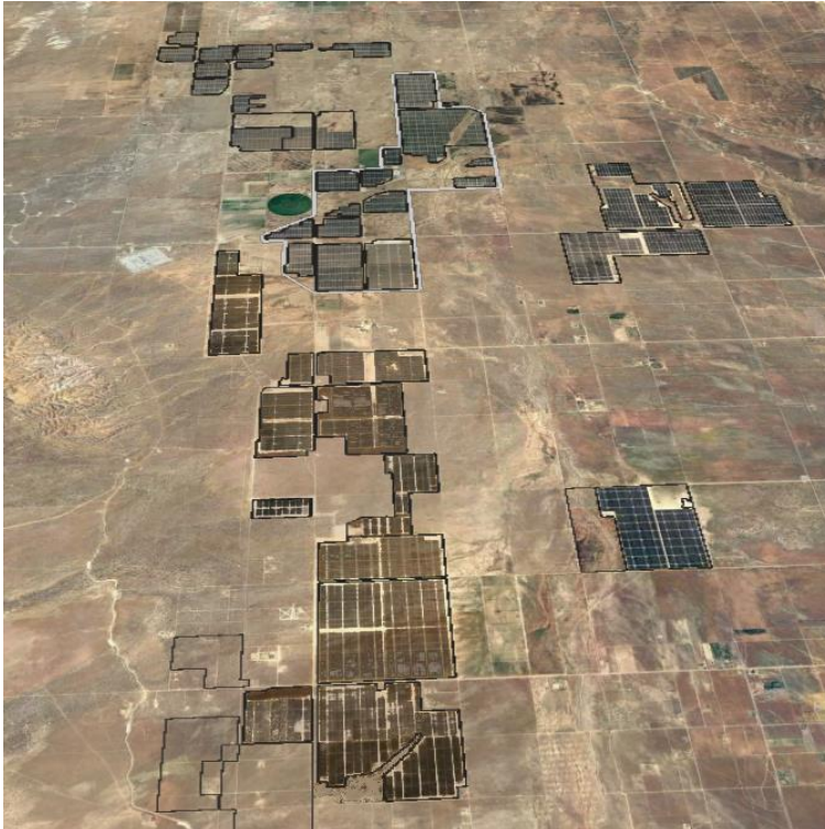
The central Antelope Valley (viewed towards the East) contains many solar arrays. The group of plots within the light grey border near the top are the 585 MW Solar Star project - for a time the world's largest single plant.
