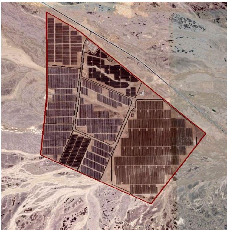
A compact example of a Solar Park is at Ma'an in southern Jordan, which contains 9 plants with a total capacity of about 200 MW.
